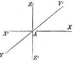
horizontal, and to intersect ZAX in the horizontal line X'X. The plane YAZ is perpendicular to the other two planes and intersects the horizontal plane in the horizontal line YY', and the vertical plane in the vertical line ZZ'. The three planes are called, the co-ordinate planes.
